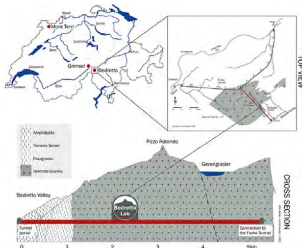
Image: Location of the BedrettoLab. © Swiss Seismological Service at ETH Zurich, 2020.
