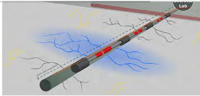
Image: The multi packer system in the BedrettoLab. [Click on the image to see more details.](#)
